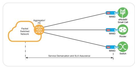
As a service demarcation device, it can attach Service VLAN and add priority marking to multiple services at the customer premises, ensuring proper service handling throughout the service provider network.
